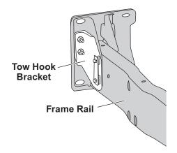
3. Install the mount by holding the front portion of the mount in place and securing with the previously removed bumper bracket bolt assembly. Clamp the rear portion of the mount into position on the truck frame, making sure the mount is tight against the bottom of the frame.
